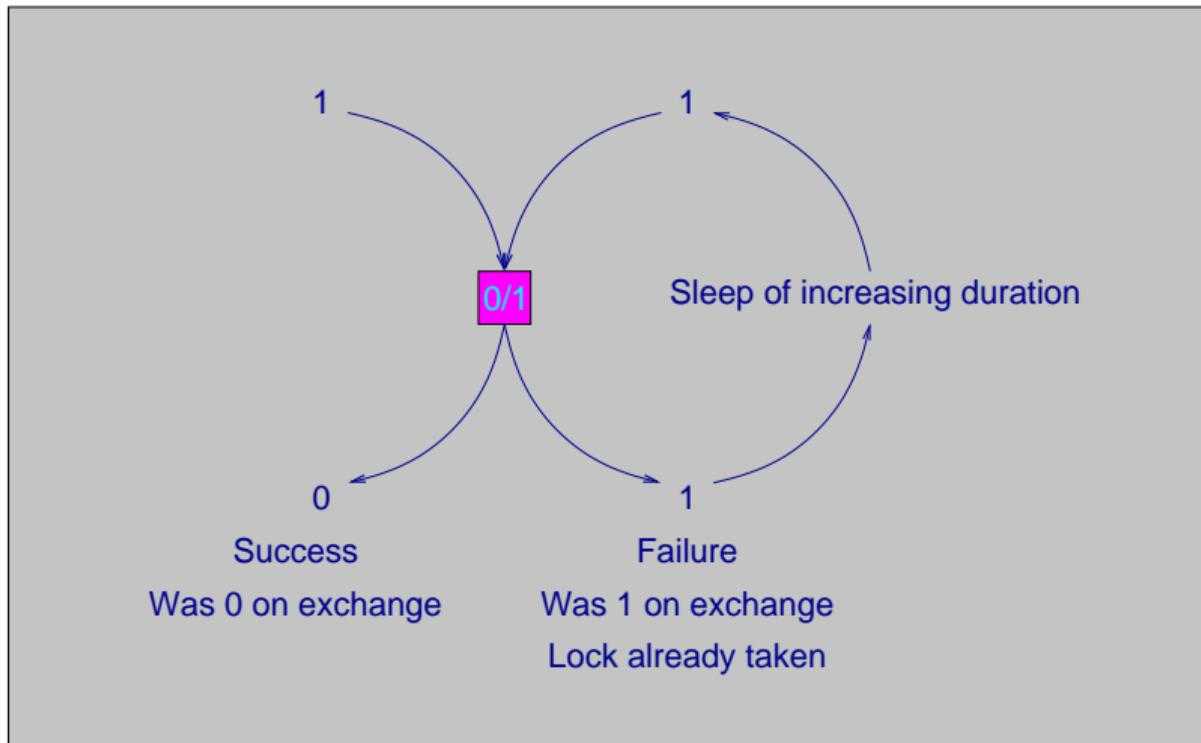
Spinlocks are designed for short-lived locking operations, like access to control structures. They are not be used to protect code that makes kernel calls or other heavy operations.
