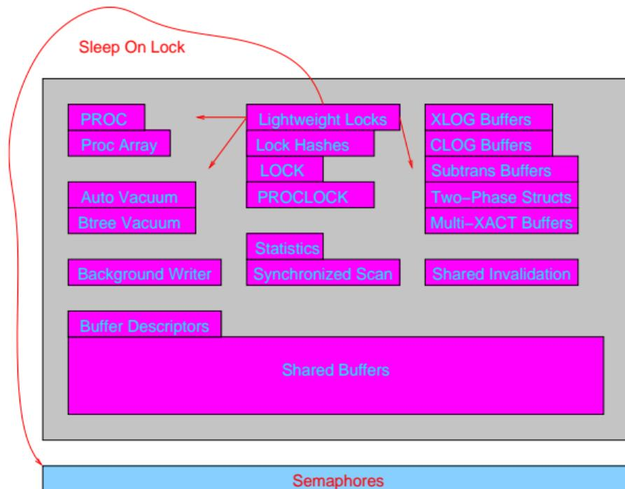
Light weight locks attempt to acquire the lock, and go to sleep on a semaphore if the lock request fails. Spinlocks control access to the light weight lock control structure.
